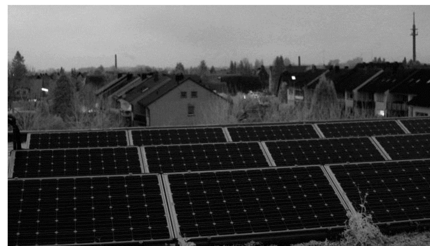
Fig. 8: EL exposure with extraneous light at dawn without current feeding
